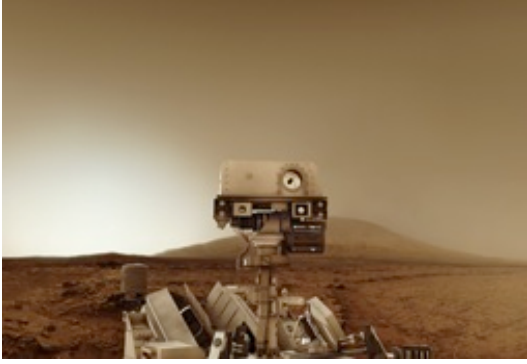
Image 37 – Mars Curiosity Rover 2 The Mars Rover uses cameras, drills, x-rays and lasers to examine the surface of Mars. Copyright: 2016 December Media
